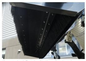
The suction head effectively collects leaves from the pitch without removing granulate from the bottom of the field.
